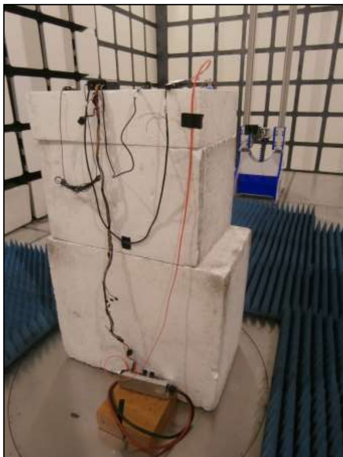
Figure 26 – Test Setup – 1 GHz to 18 GHz, X Orientation
