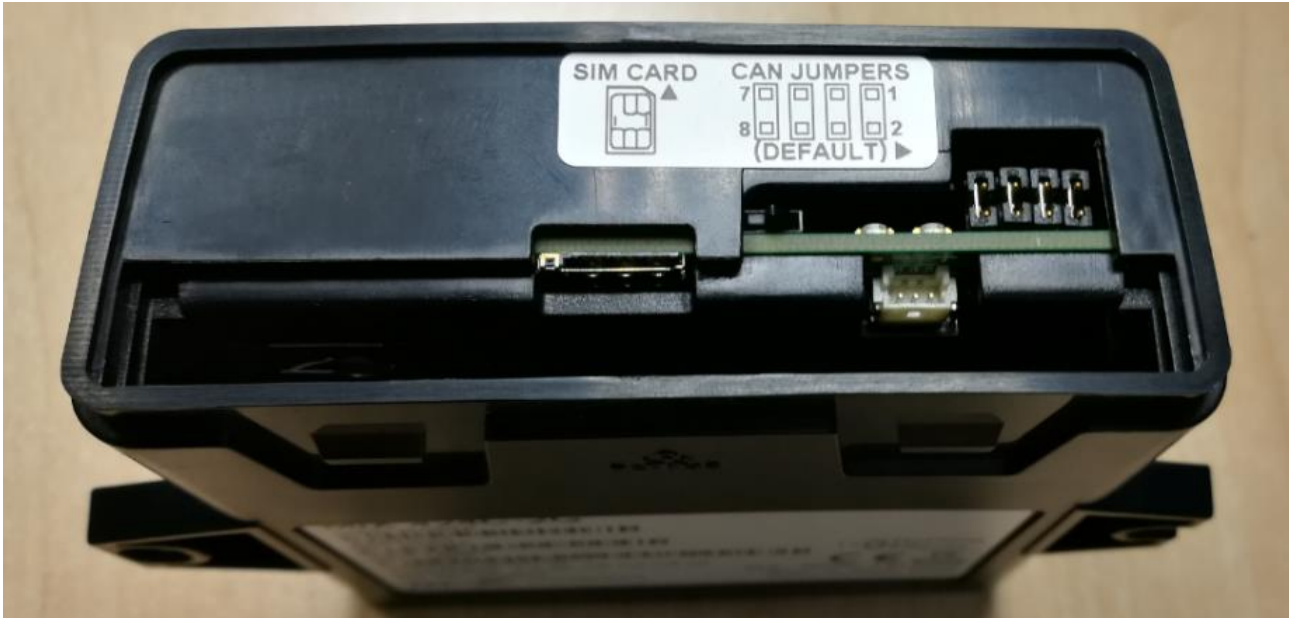
Figure 1: Picture of the MiX 45MC-4G (back plate removed)
