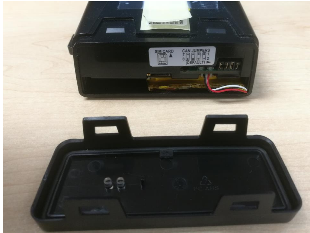
Figure 3: View of MiX 45MC-4G-B with Rear Panel Removed (backup battery inserted)
