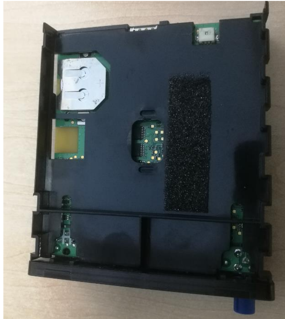
Figure 6: Bottom Side of Main PCB on Carrier – battery NOT fitted (MiX 45MC-4G)
