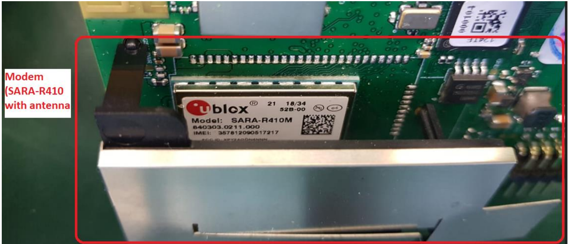
Figure 10: View of Modem plus Antenna on Main PCB
