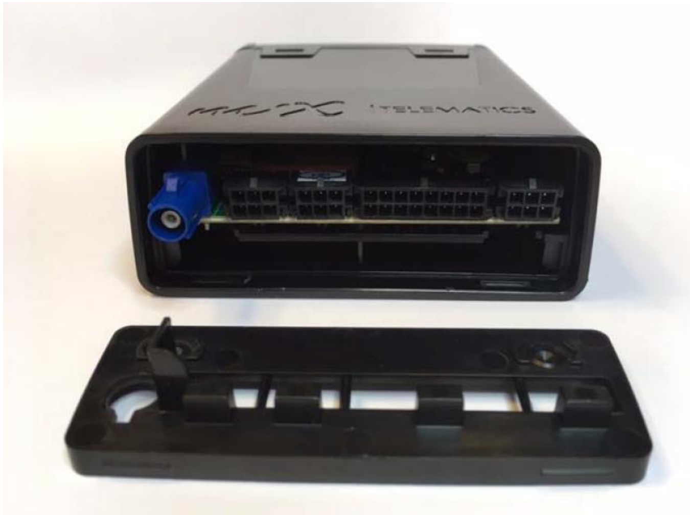
Figure 1: View of MiX 45MC-4G/MiX 45MC-4G-B with Front Panel Removed
