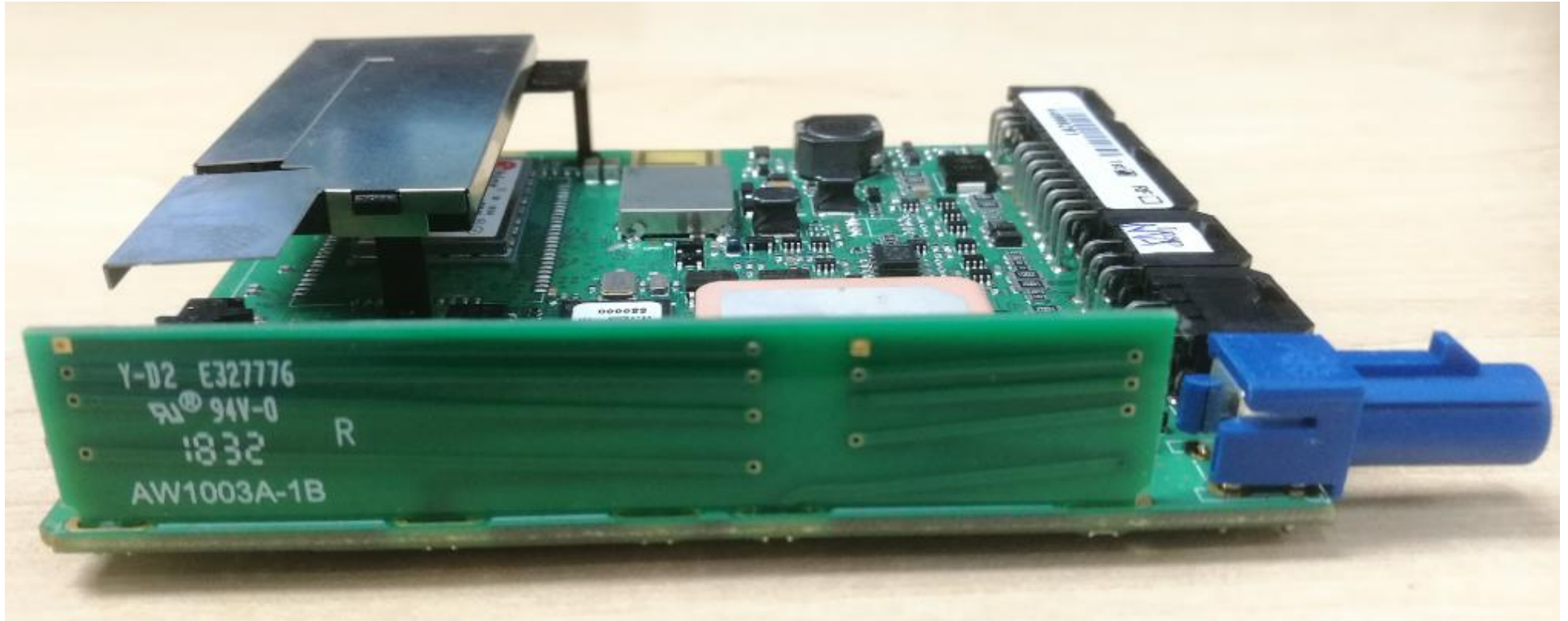
Figure 8: Side View of Main PCB showing 434 & 915 MHz Antenna
