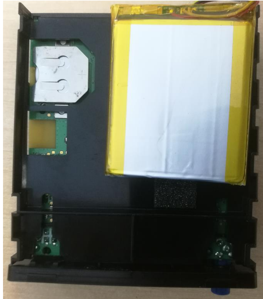
Figure 6: Bottom Side of Main PCB on Carrier with battery fitted (MiX 45MC-4G-B)
