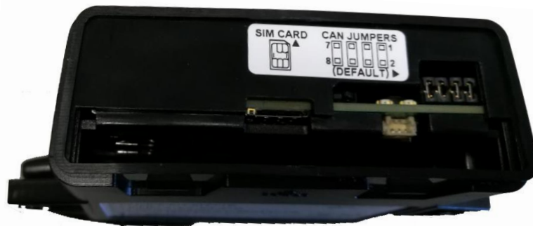
Figure 7: Position of jumpers on the PCB.
