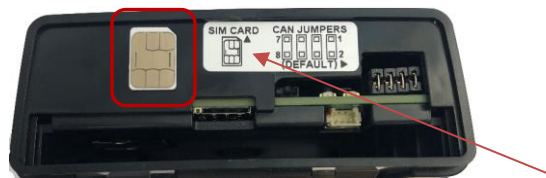
Figure 3: Position the SIM as shown on the unit.
