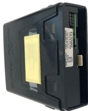
Figure 4: Insert the SIM card into SIM card slot; ensure it is fully seated (clicks into place).
