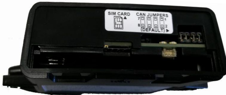
Figure 7: Position of jumpers on the PCB.
