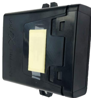
Figure 5: Clip the cover back on; the hooks need to click into place.
