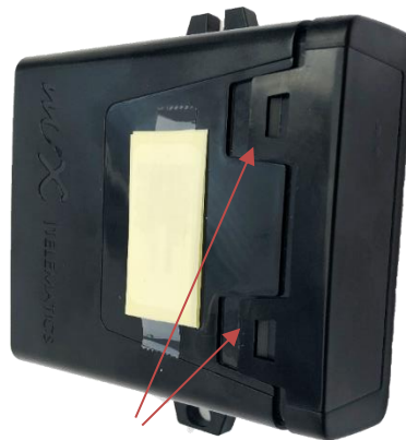
Figure 1: Opening of side clips
