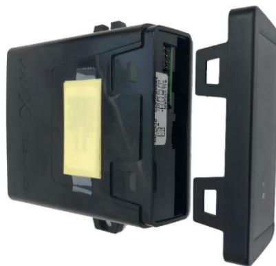
Figure 2: Unhook the cover
