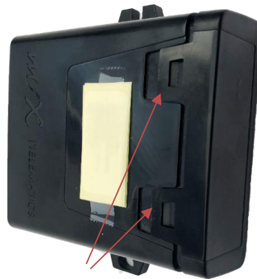
Figure 1: Opening of side clips
