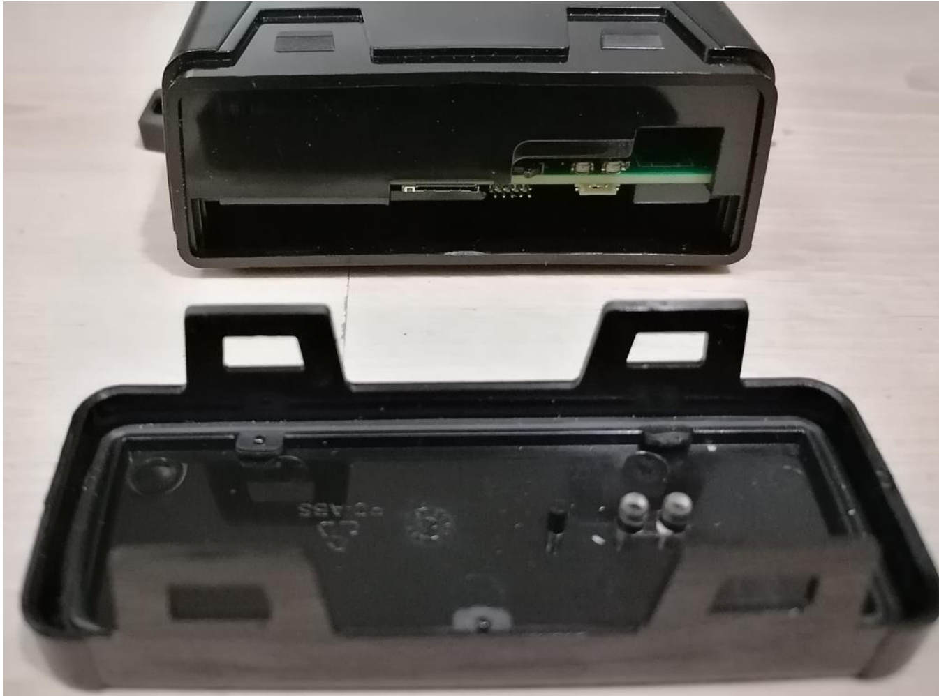
Figure 8: View of MiX 4401 with Rear Panel Removed
