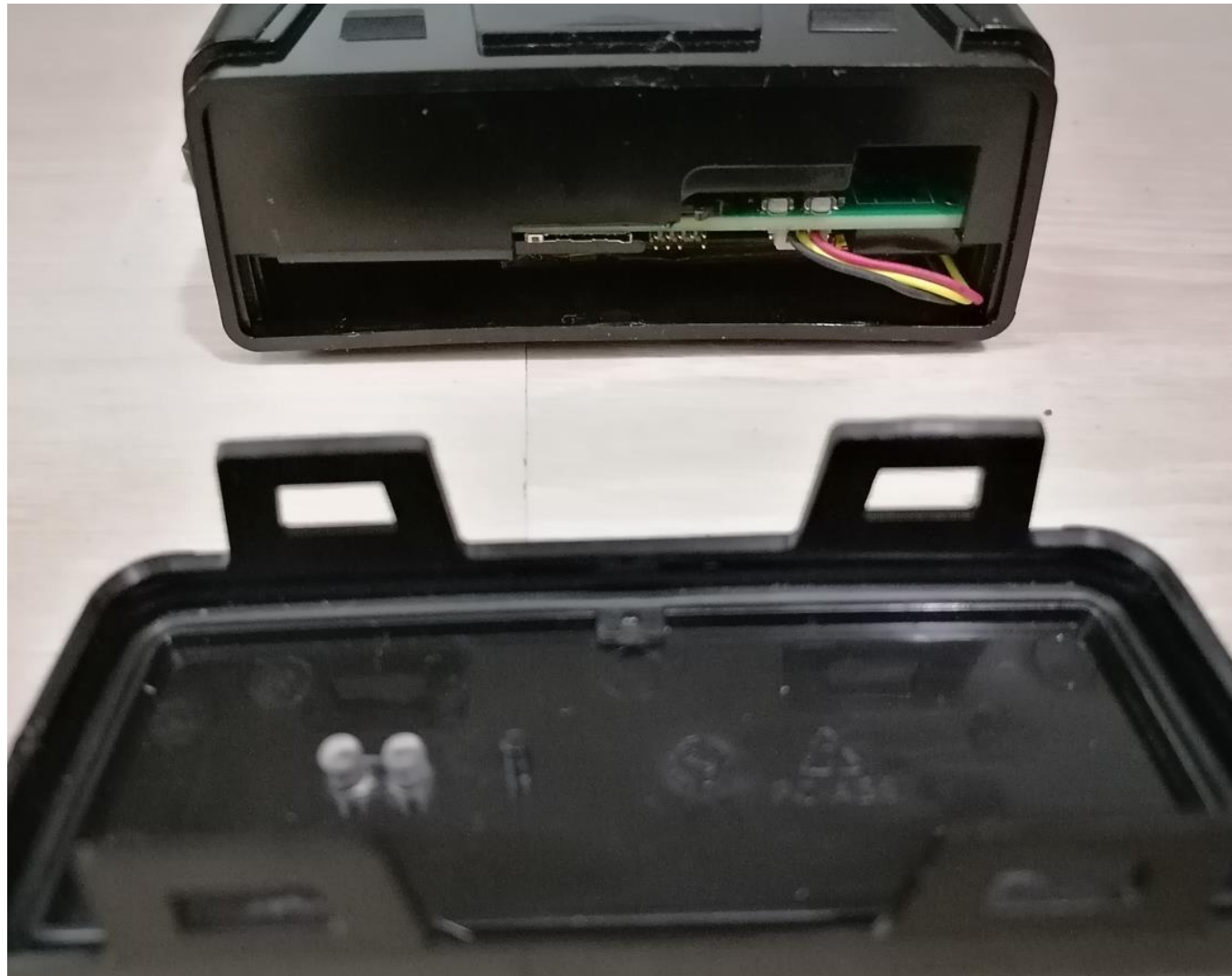
Figure 3: View of MiX 4401-B with Rear Panel Removed (backup battery inserted)
