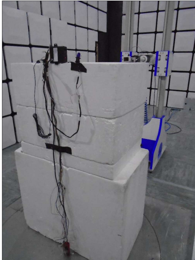
Figure 74 - Test Setup - 18 GHz to 25 GHz - Z Orientation
