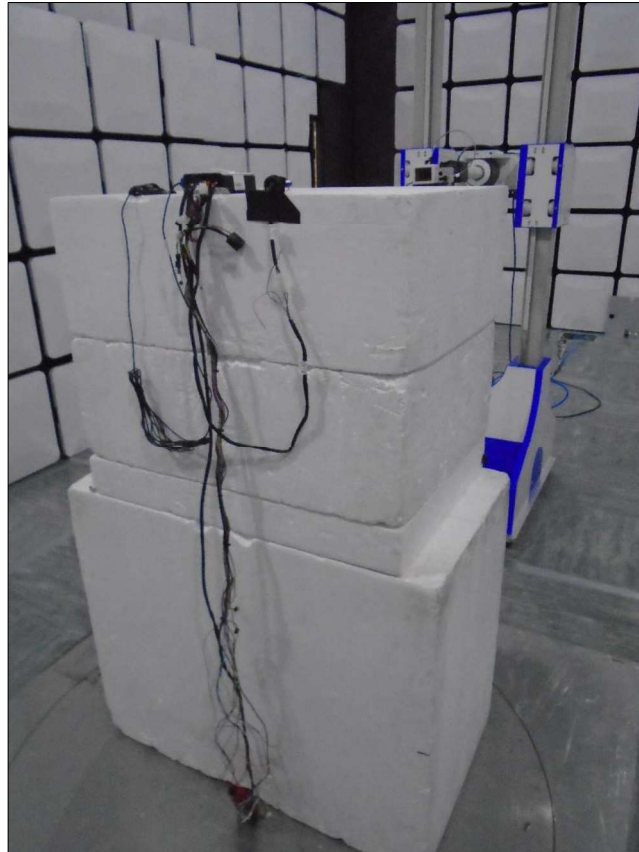
Figure 72 - Test Setup - 18 GHz to 25 GHz - X Orientation
