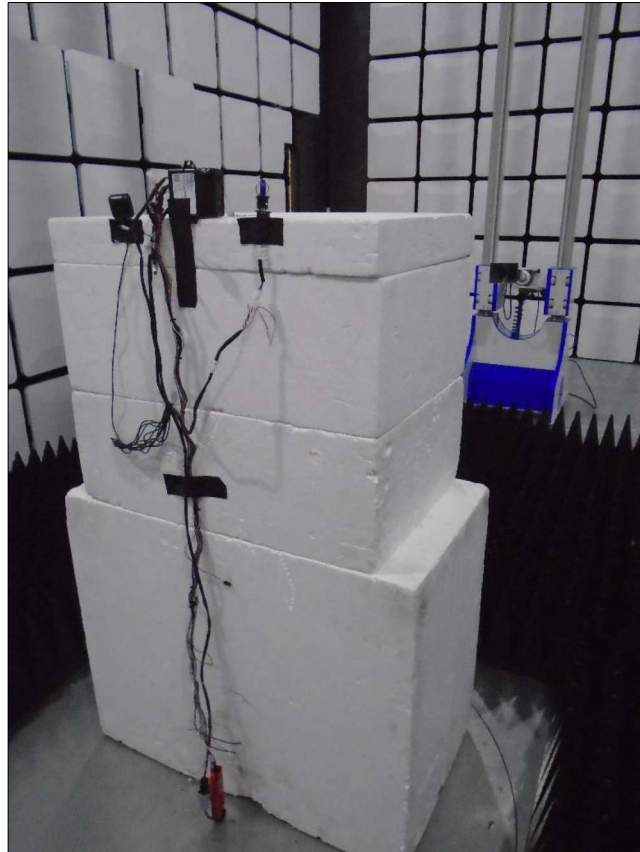
Figure 71 - Test Setup - 1 GHz to 18 GHz - Z Orientation
