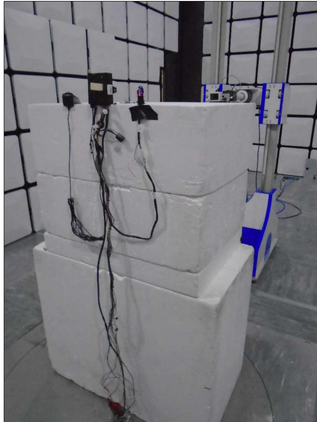
Figure 73 - Test Setup - 18 GHz to 25 GHz - Y Orientation
