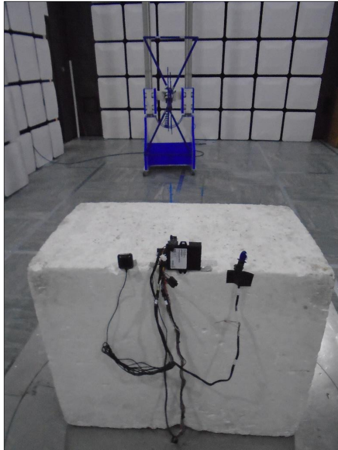
Figure 68 - Test Setup - 30 MHz to 1 GHz - Z Orientation
