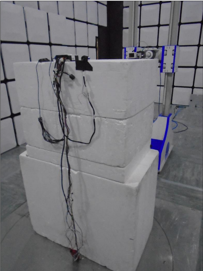
Figure 72 - Test Setup - 18 GHz to 25 GHz - X Orientation
