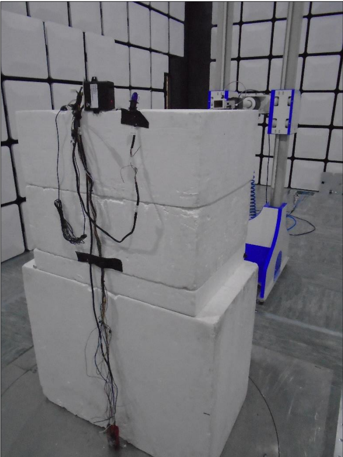
Figure 74 - Test Setup - 18 GHz to 25 GHz - Z Orientation
