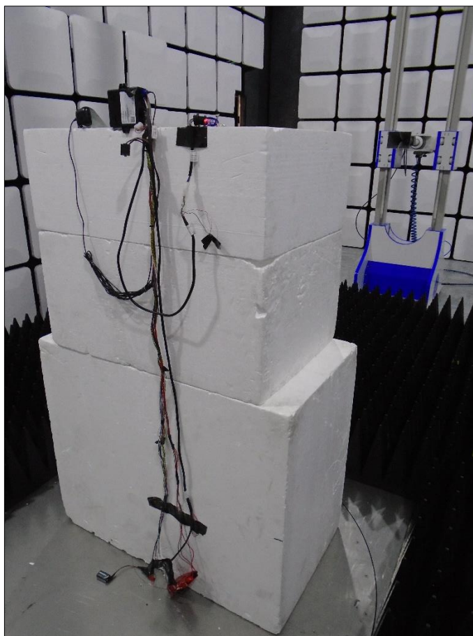
Figure 50 - Test Setup - 1 GHz to 18 GHz - Z Orientation
