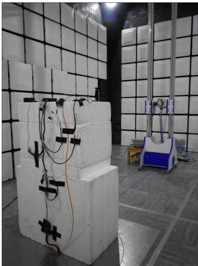
Figure 51 - Test Setup - 18 GHz to 25 GHz - X Orientation
