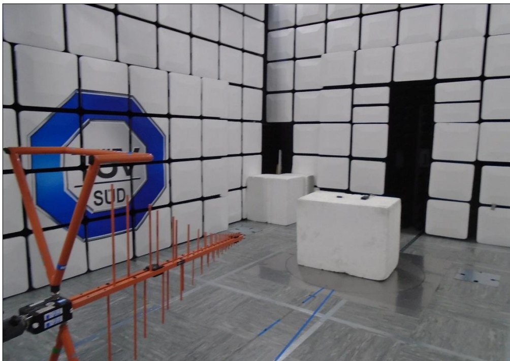
Figure 19 - Test Setup - 30 MHz to 1 GHz
