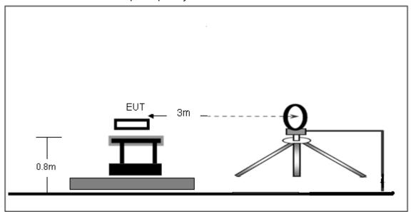
(B) Radiated Emission Test-Up Frequency 30MHz~1GHz
