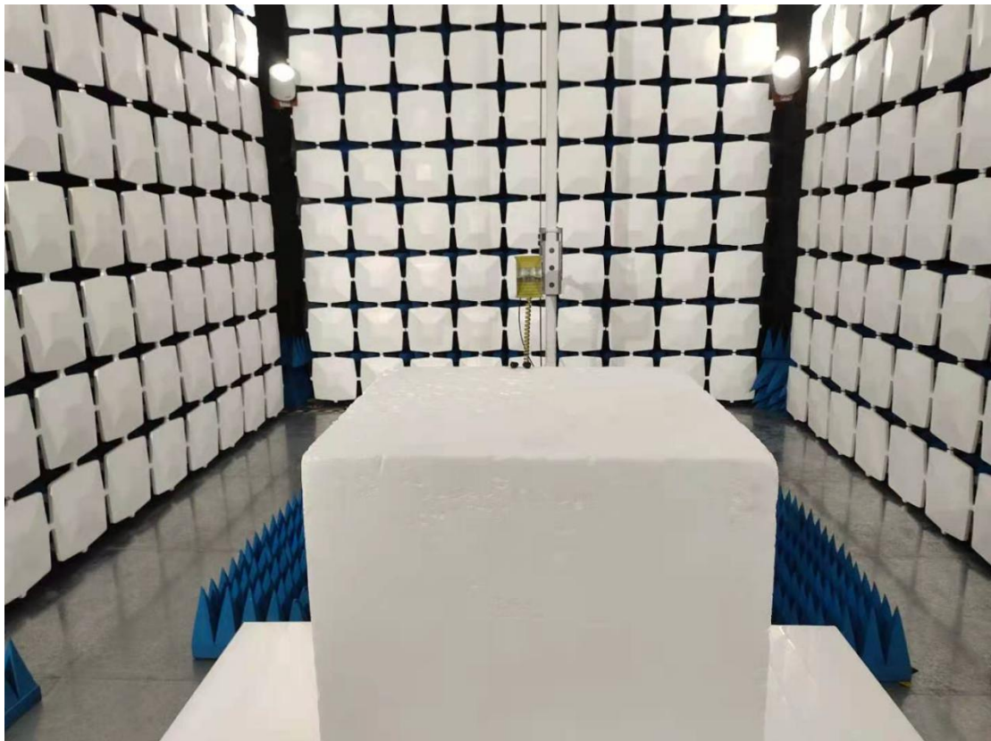
Above 1GHz for radiated emission test setup
