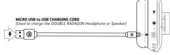
The Double Radagon Headphone & Speaker will show a red LED when charging. LEDs will turn off when Double Radagon Headphone & speaker are fully charged.
