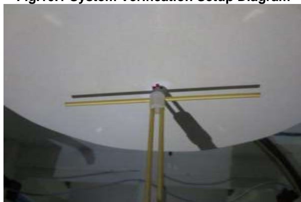
Fig.10.2 Photo of Dipole setup
