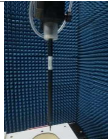
Fig.8.2 Photo of E-Field Probe
