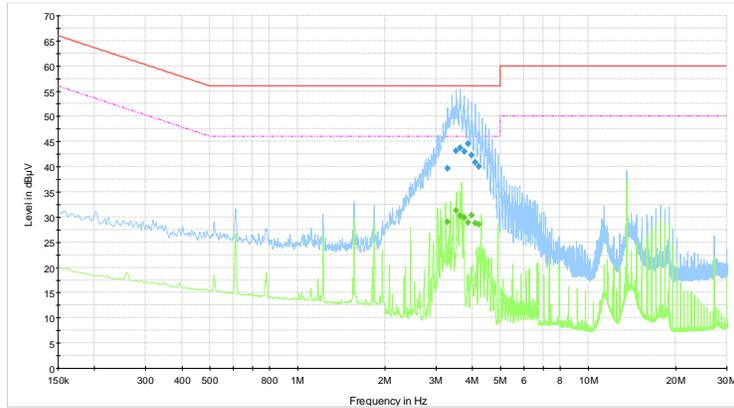
SR299005.CE-240V-port relay-L1-tx on with dummy load
