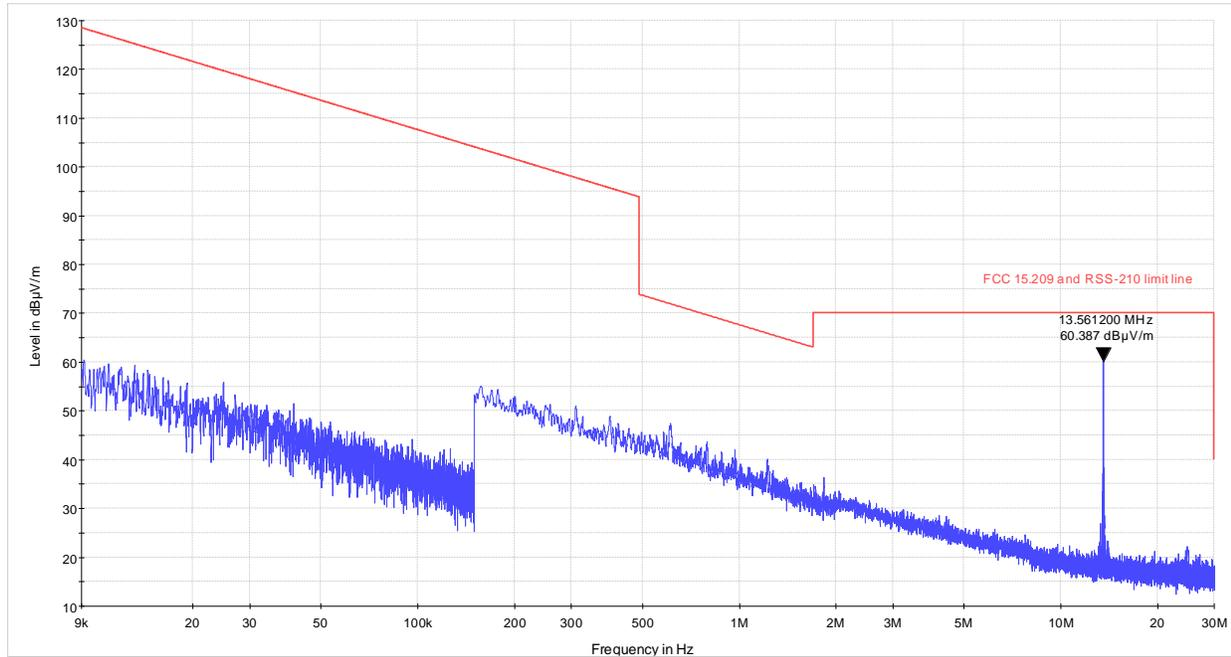
Figure 8.4-1: Field strength of spurious emissions below 30 MHz
