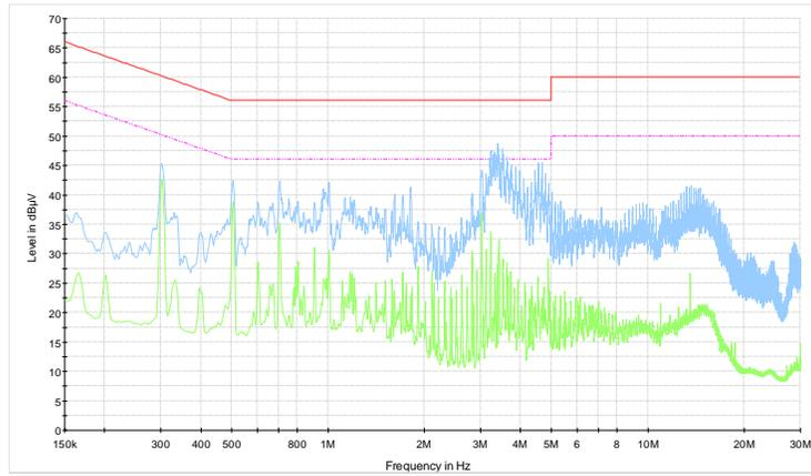
5W 299005 CE-120Vvac, input-port AA128-L1-tx-on-with dummy load
