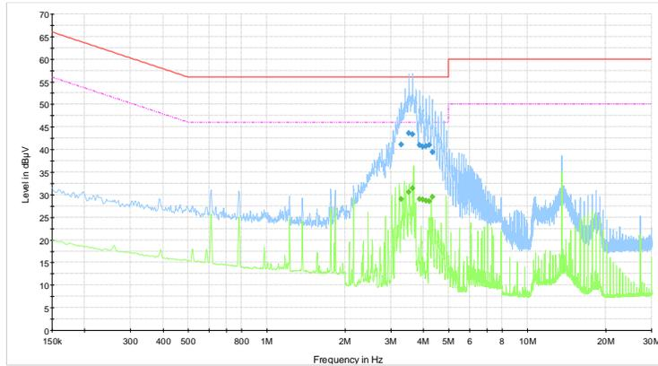
SR299005.CE-120V-portrelay-L1-tx on with dummy load
