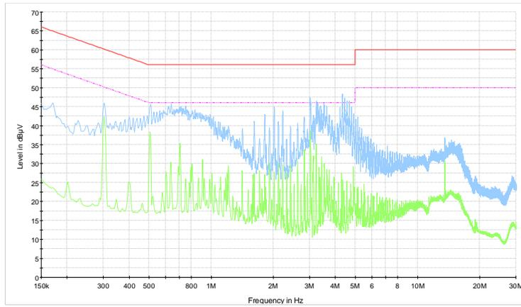
5W 299005.CE-240V-port AA128-L1-tx on with dummy load
