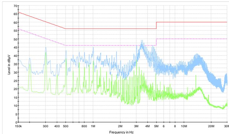
5W 299005 CE-120V-port AA128-N-tx-on-with dummy load
