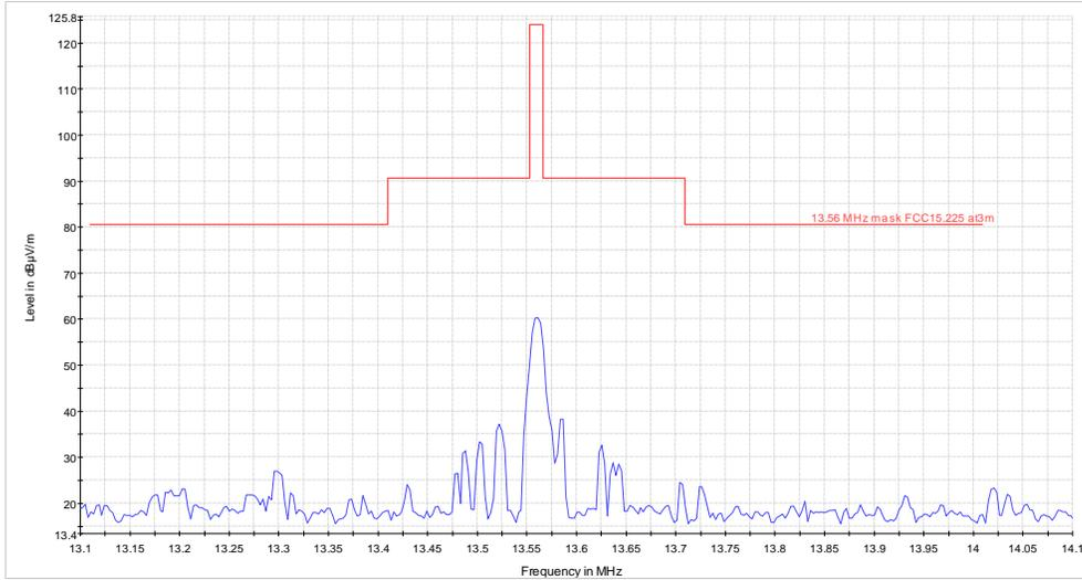
Figure 8.3-2: Field strength within 13.11–14.01 MHz band
