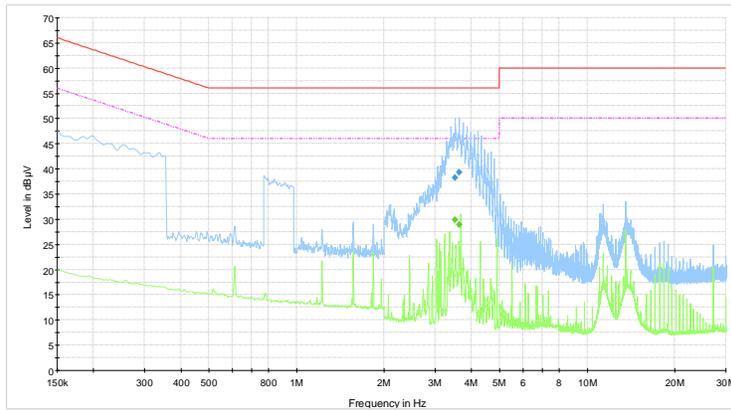
SR299005.CE-240V-port relay-N1-tx on with dummy load
