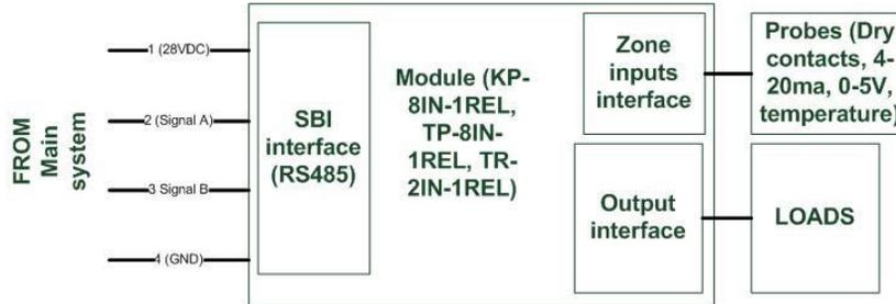
Figure 1 : Network definition between the main system and the external module
