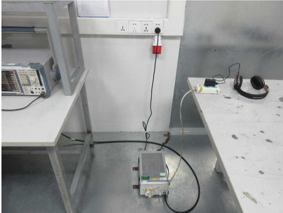
Photo of Conducted Emission Measurement
