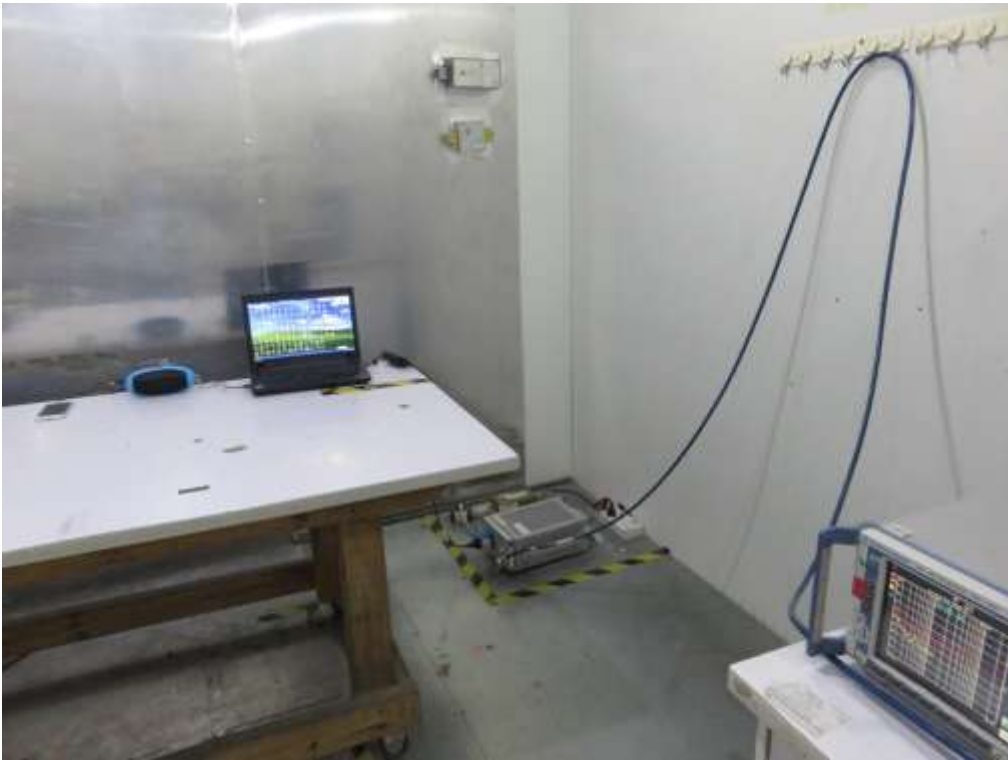
FCC RADIATED EMISSION TEST SETUP
