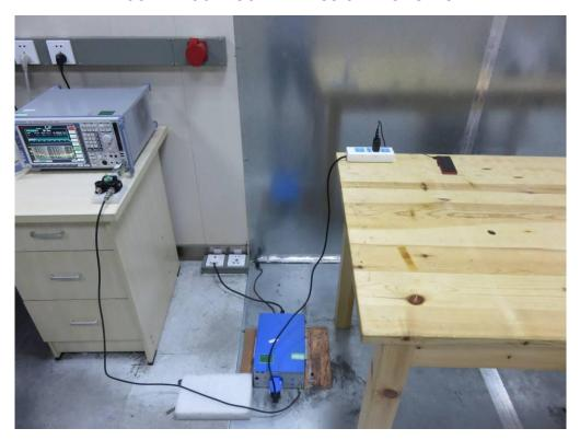
FCC RADIATED EMISSION TEST SETUP
