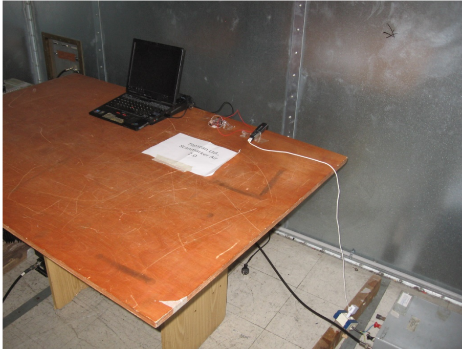
Figure 3. Conducted Emission from AC Power Line Test
