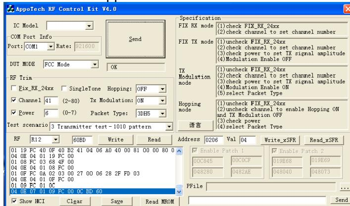
The test software was used to control EUT work in continuous TX mode, and select test channel, Wireless mode as below table
