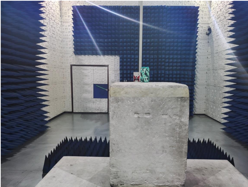
RADIATED EMISSION TEST SETUP ABOVE 1GHZ
