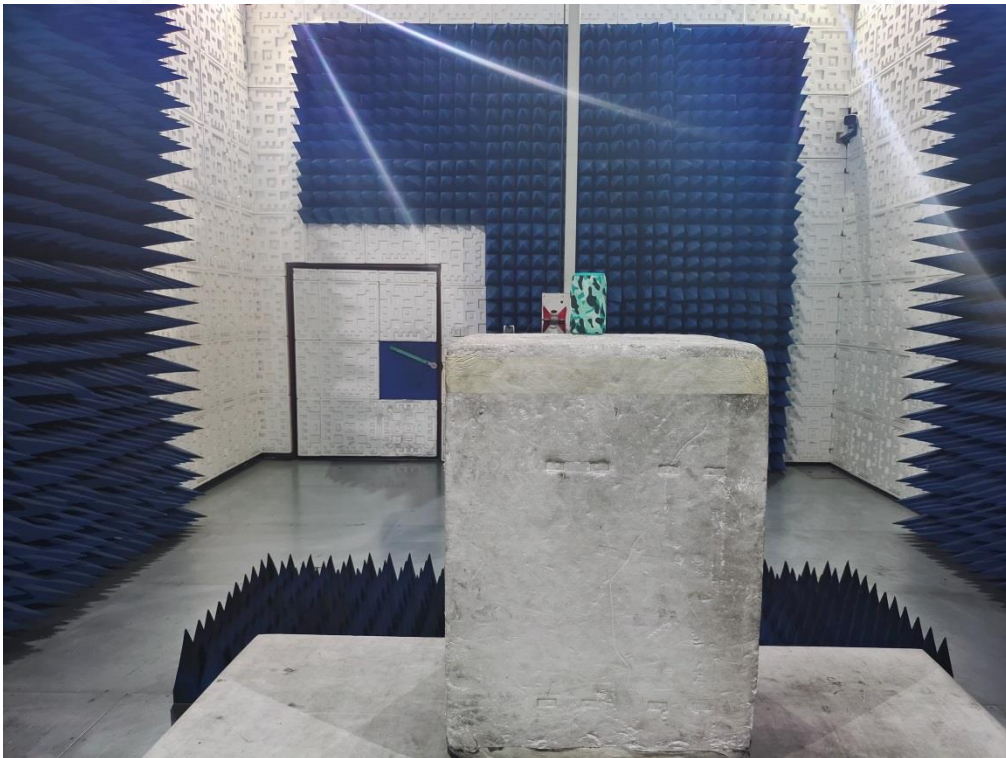
RADIATED EMISSION TEST SETUP ABOVE 1GHZ
