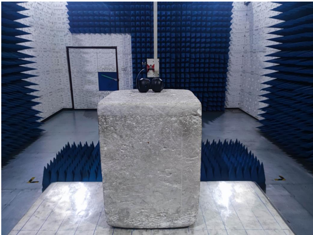
RADIATED EMISSION TEST SETUP ABOVE 1GHz
