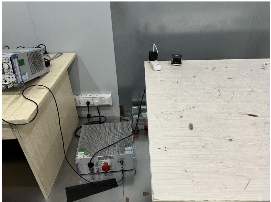
Conducted Emission Test Setup
