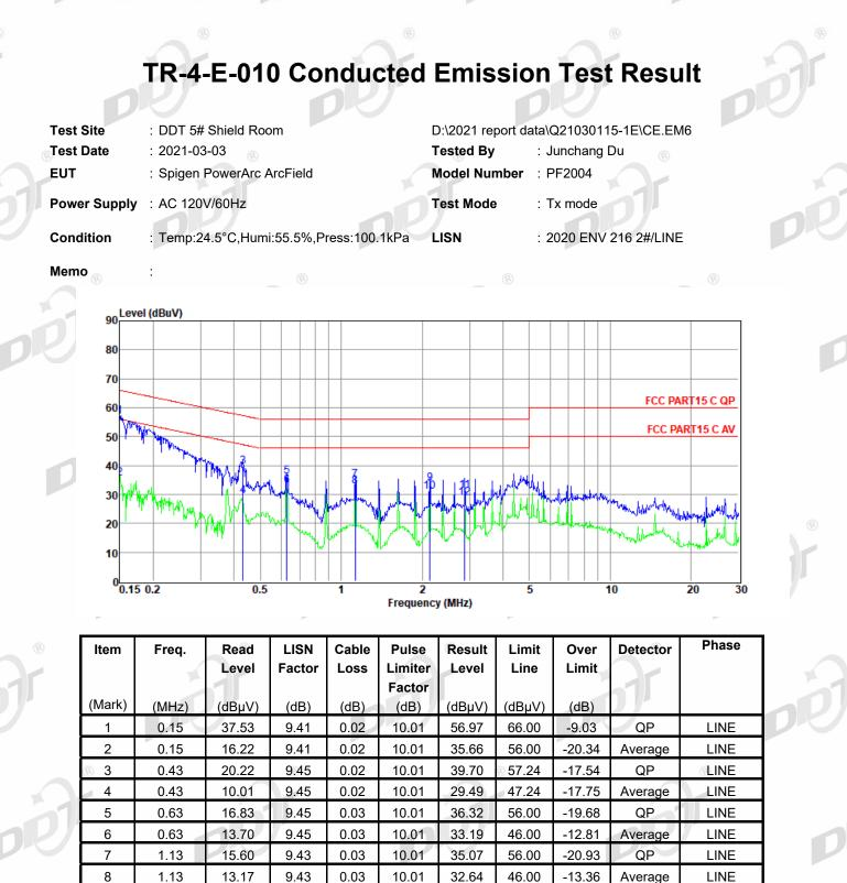
1. Result Level = Read Level +LISN Factor + Pulse Limiter Factor + Cable loss.
