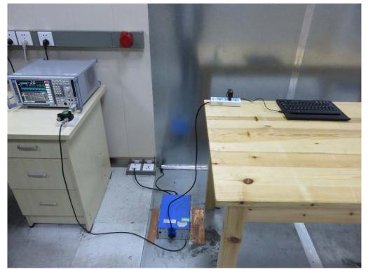
FCC RADIATED EMISSION TEST SETUP
