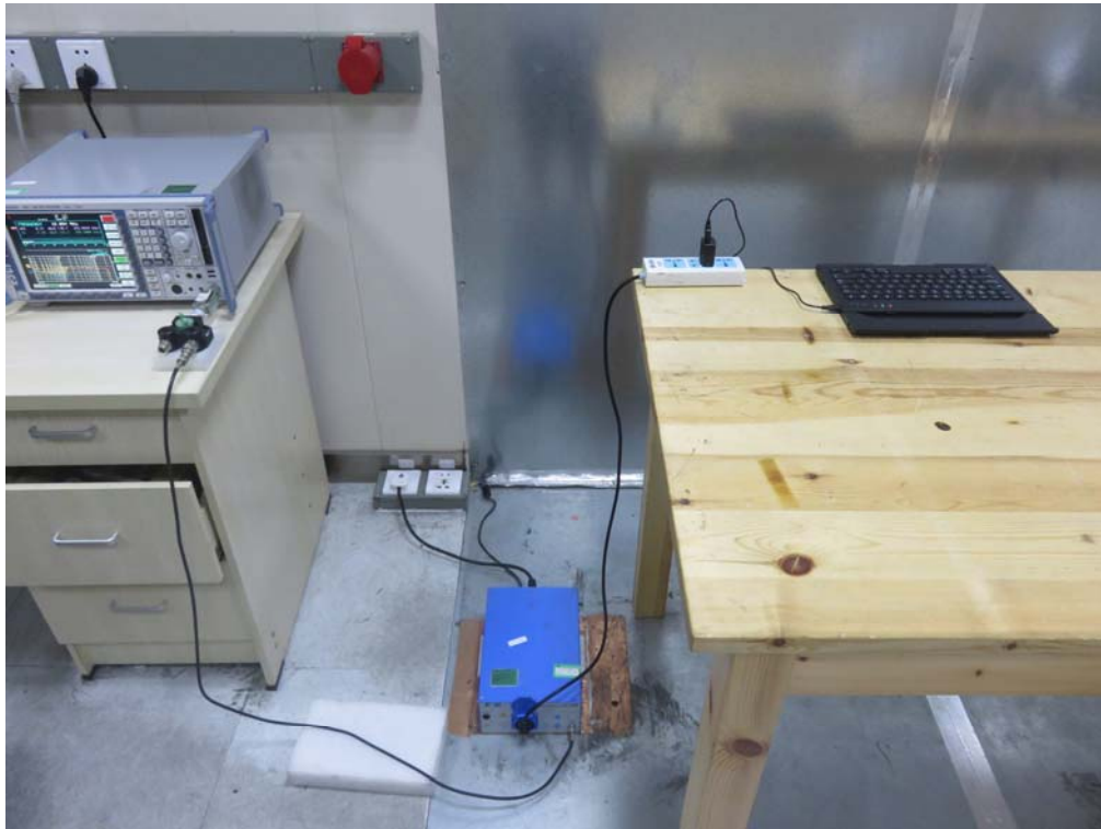
FCC RADIATED EMISSION TEST SETUP
