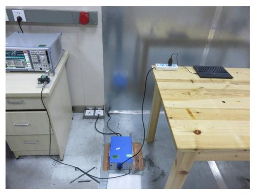
FCC RADIATED EMISSION TEST SETUP
