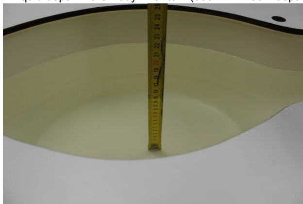
Liquid depth in the Body Phantom (1800 MHz 15cm depth)
