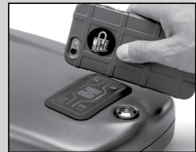
One to five RFID tags can be programmed into the safe.
