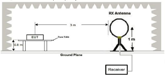
2. Radiated Emission Test-Up Frequency 30MHz~1GHz
