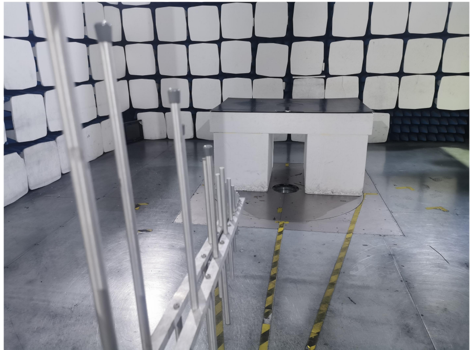
Radiation Emission Test Setup (30MHz to 1GHz)
