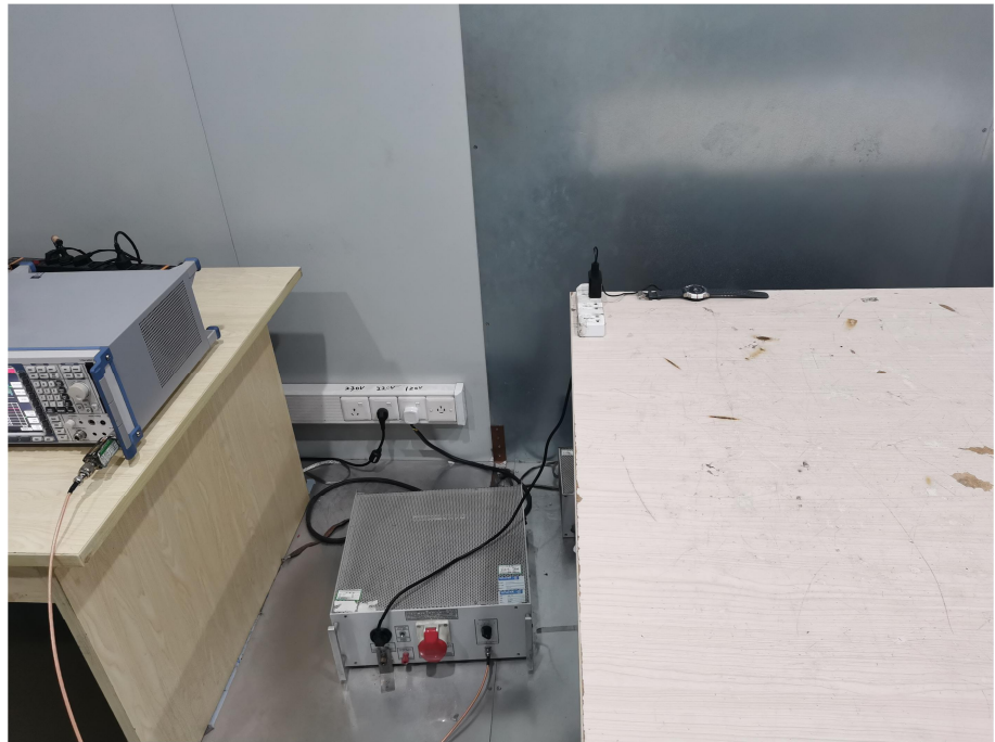
Conducted Emission Test Setup
