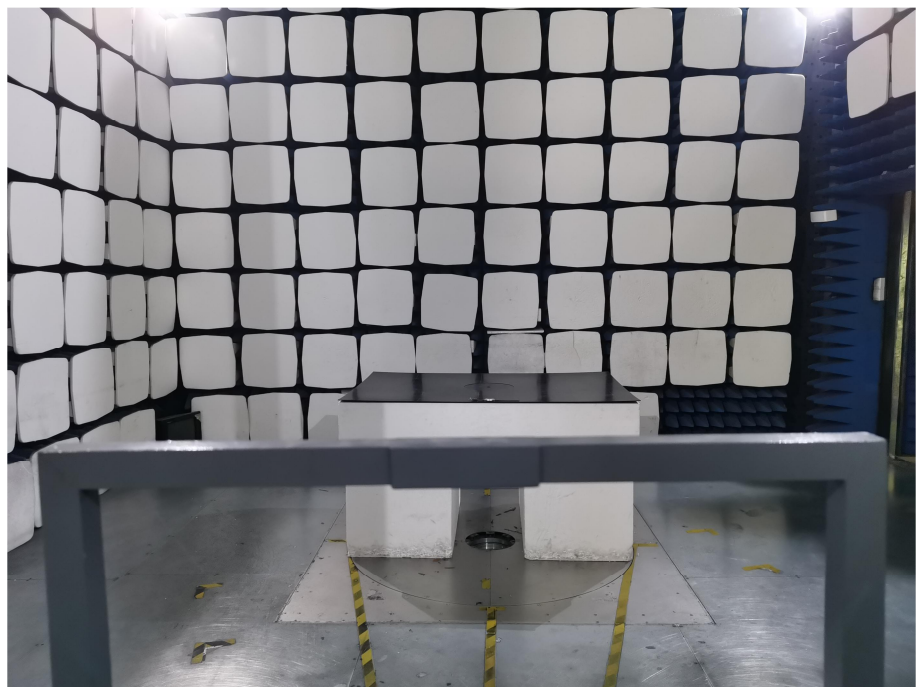
Radiation Emission Test Setup (Below 30MHz)
