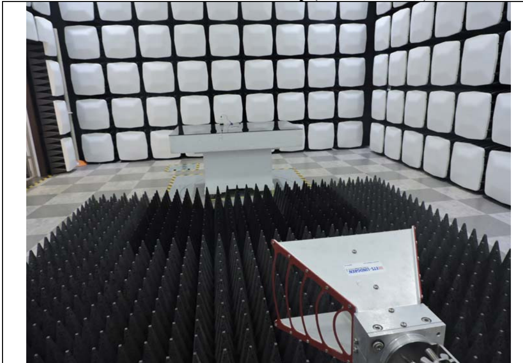
Radiated Emission Test Setup (ABOVE 1 GHz)
