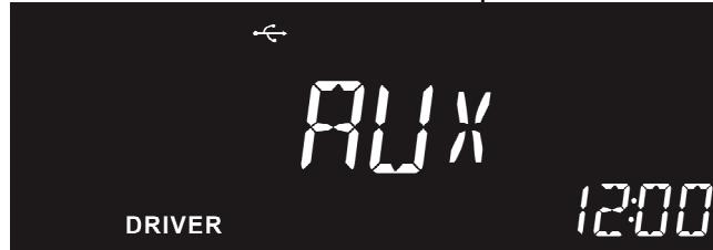
Notice: Radio can turn to AUX play mode whether there is a AUX device in or not. Please make sure the AUX device is in on mode otherwise there is no sound.
