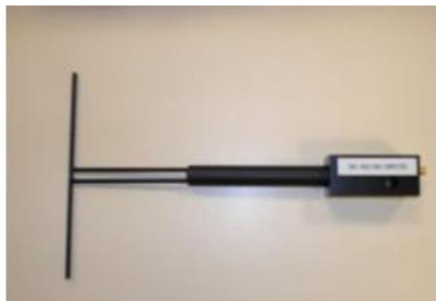
Figure 1 – Satimo COMOSAR Validation Dipole
