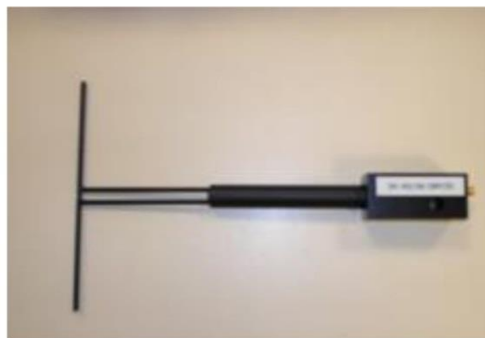
Figure 1 – Satimo COMOSAR Validation Dipole
