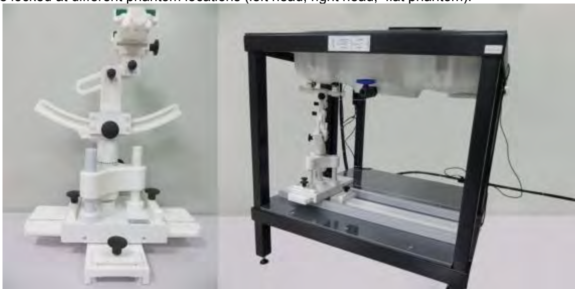
Device holder supplied by SATIMO
