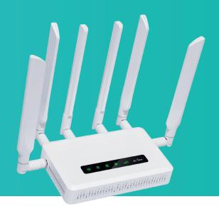
GL-X3000 is a Wi-Fi 6 4G/5G Cellular Router designed to offer internet speed of 574Mbps (2.4GHz) and 2402Mbps (5GHz), with a combined maximum Wi-Fi speed of 3000Mbps. It is designed for high-speed internet usage with a failover cellular connection, or for scenarios without a reliable source of internet, including recreational vehicles traveling in remote locations, or public transport within high interference city limits.
