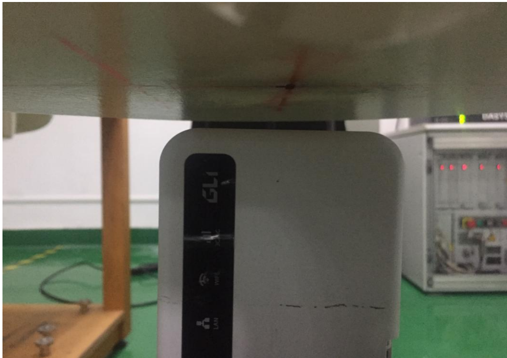
10mm Body-worn bottom Side Setup Photo
