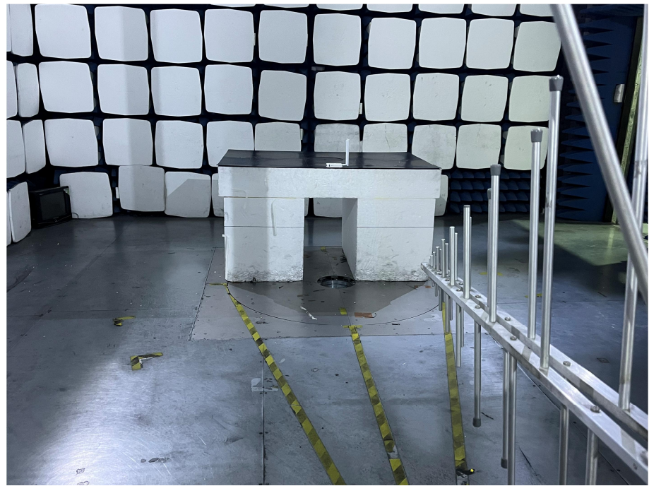
Radiation Emission Test Setup (30MHz to 1GHz)
