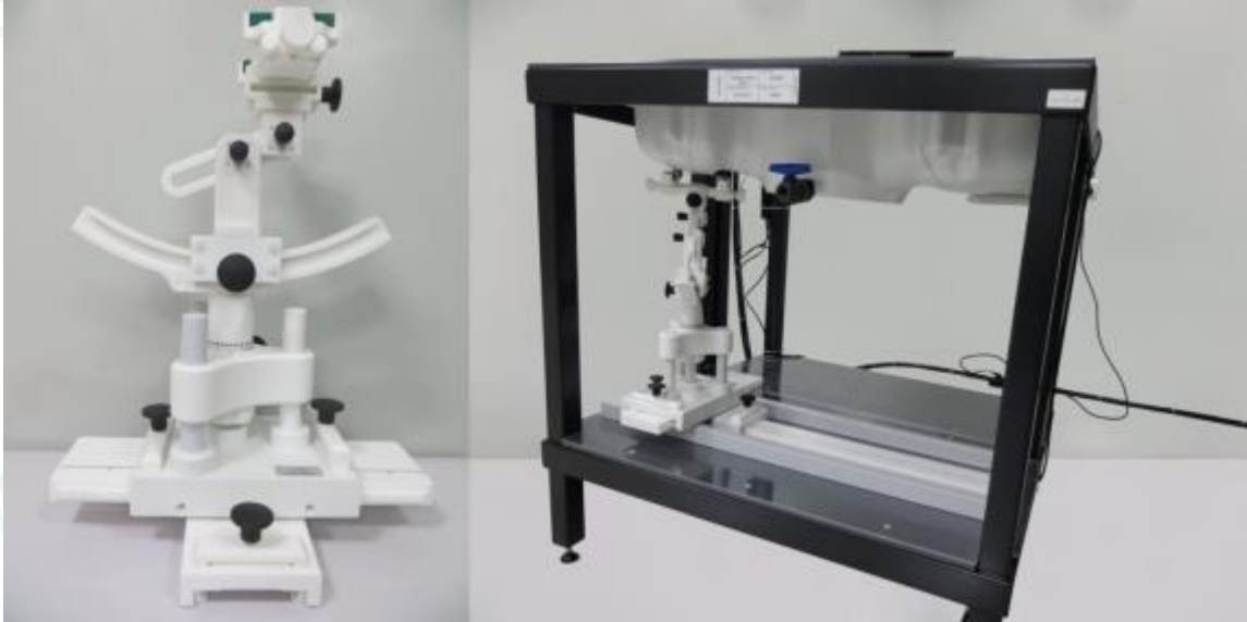
Device holder supplied by SATIMO
