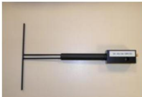
Figure 1 – Satimo COMOSAR Validation Dipole
