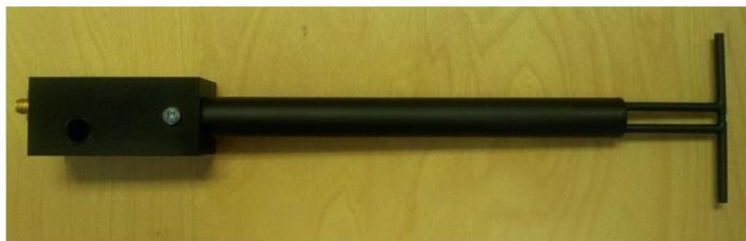
Figure 1 – MVG COMOSAR Validation Dipole
