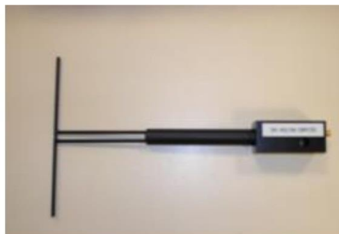
Figure 1 – Satimo COMOSAR Validation Dipole
