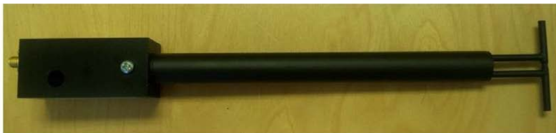
Figure 1 – MVG COMOSAR Validation Dipole
