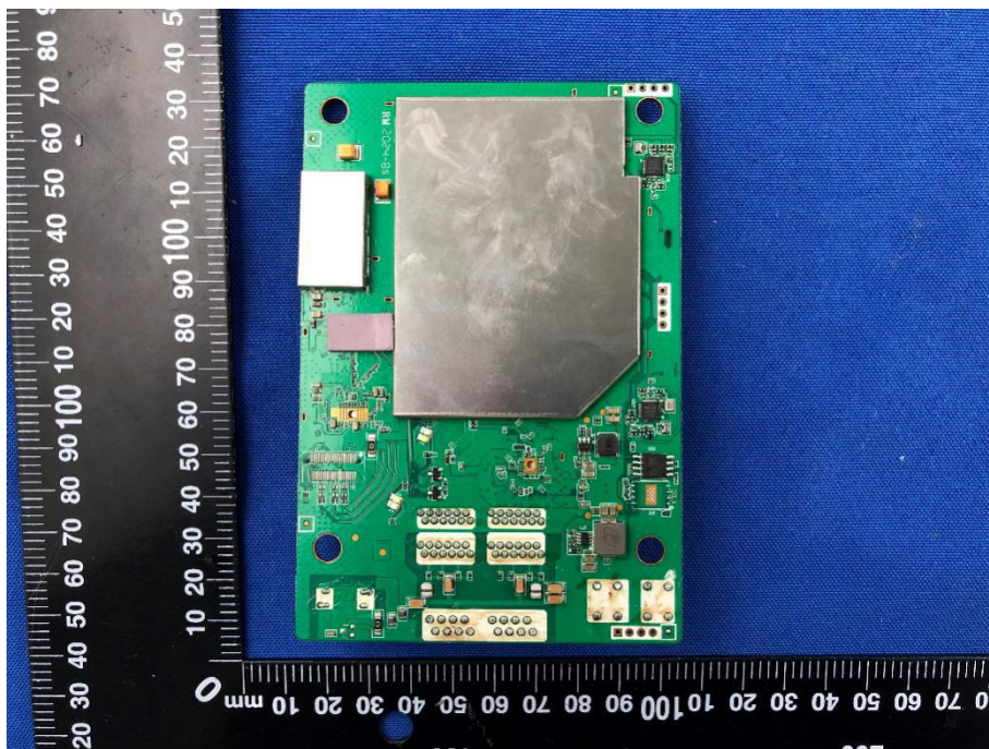
MAIN BOARD BACK VIEW (WITH SHIELDING)
