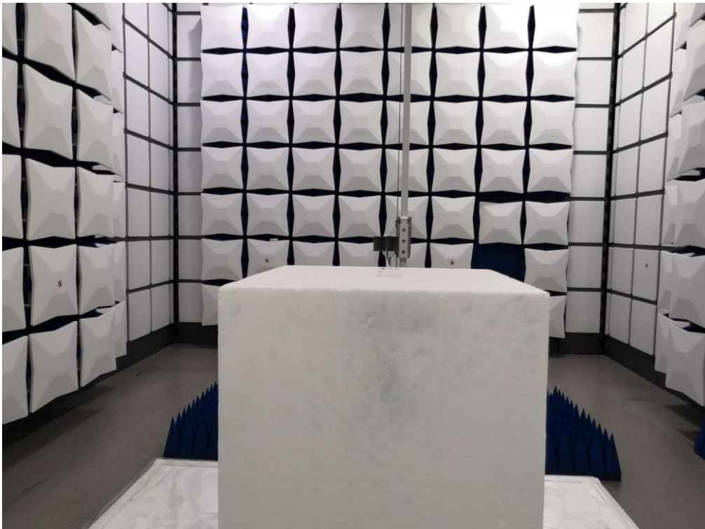
FCC RADIATED EMISSION TEST SETUP ABOVE 1GHZ
