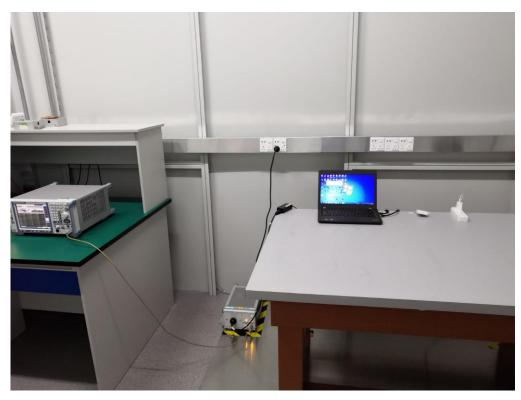
FCC RADIATED EMISSION TEST SETUP BELOW 1GHZ
