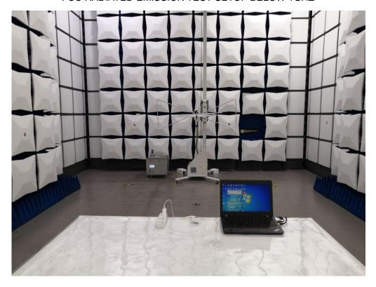
FCC RADIATED EMISSION TEST SETUP ABOVE 1GHZ
