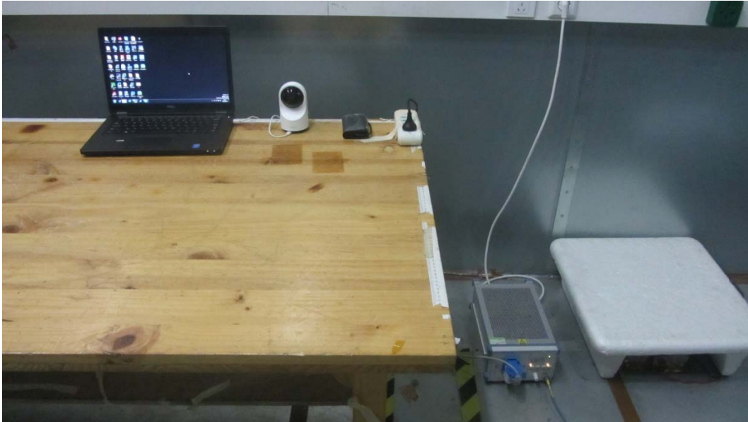
Picture 3 Conducted Emission Test Setup
