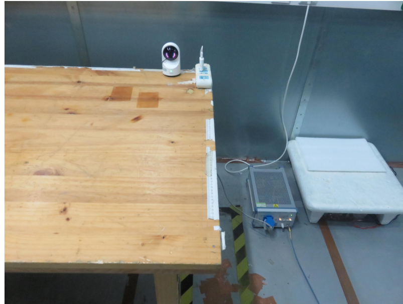
Picture 3 Conducted Emission Test Setup
